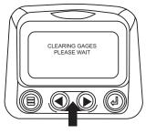
When the gage data has cleared, the display automatically returns to the "Utilities" menu. Scroll to "Software Version". Touch "Select" to view the software version currently in the diagnostic display.
